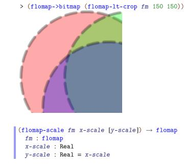
Scales *fm* to a proportion of its size. Uses bilinear interpolation to sample between integer coordinates, and reduces resolution (blurs) correctly before downsampling so that shrunk images are still sharp but not aliased (pixelated-looking).
