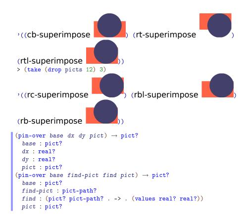
Creates a pict with the same bounding box, ascent, and descent as *base*, but with *pict* placed on top. The *dx* and *dy* arguments specify how far right and down the second pict's corner is from the first pict's corner. Alternately, the *find-pict* and *find* arguments find a point in *base* for *find-pict*; the *find* procedure should be something like lt-find.
