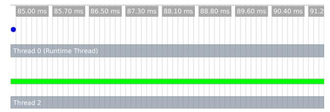
Notice that only one green bar is shown here because one of the mandelbrot computations is not being evaluated by a future (on the runtime thread).
