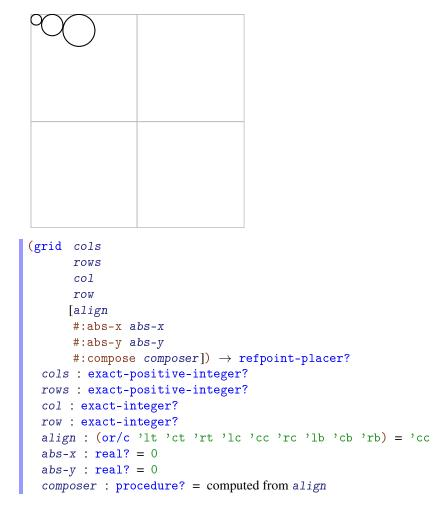
Returns a placer that places picts according to a position in a virtual grid. The *row* and *col* indexes are numbered starting at 1.
