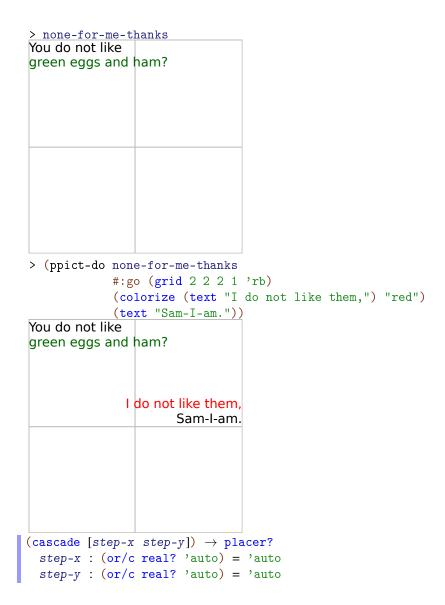
Returns a placer that places picts by evenly spreading them diagonally across the base pict in "cascade" style. This placer does not support changing the spacing by including a real number within the pict sequence.
