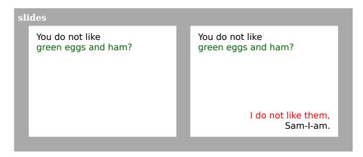
Note that the text is not flush against the sides of the slide, because pslide uses a base pict the size of the client area, excluding the margins.
