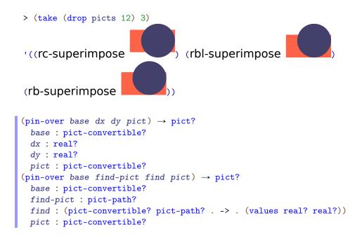
Creates a pict with the same bounding box, ascent, and descent as *base*, but with *pict* placed on top. The *dx* and *dy* arguments specify how far right and down the second pict's corner is from the first pict's corner. Alternately, the *find-pict* and *find* arguments find a point in *base* for *find-pict*; the *find* procedure should be something like *lt-find*.
