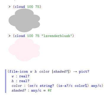
Creates a Mac-like file icon, optionally shaded. If *color* is not a string or *color*% object, it is treated as a boolean, in which case true means "gray" and false means "white".
