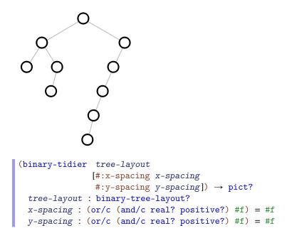
Uses the layout algorithm from *Tidier Drawing of Trees* by Edward M. Reingold and John S. Tilford (IEEE Transactions on Software Engineering, Volume 7, Number 2, March 1981) to lay out *tree-layout*.
