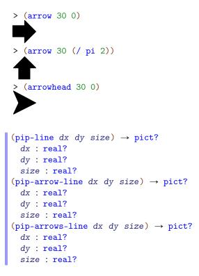
Creates a line (with some number of arrowheads) as a zero-sized pict suitable for use with pin-over. The 0-sized picture contains the starting point.
