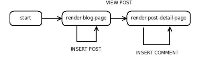
Each point in the diagram corresponds to a request-consuming handler. As we might suspect, we'll be using send/suspend/dispatch some more. Every arrow in the diagram will be realized as a URL that we generate with embed/url.
