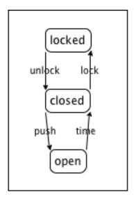
The picture displays a so-called "state machine". The three circled words are the states that our informal description of the door identified: locked, closed (and unlocked), and open.
