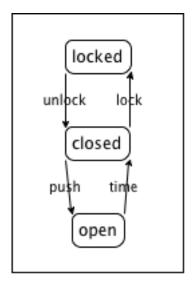
The picture displays a so-called "state machine". The three circled words are the states that our informal description of the door identified: locked, closed (and unlocked), and open. The arrows specify how the door can go from one state into another. For example, when the door is open, the automatic door closer shuts the door as time passes. This transition is indicated by the arrow labeled "time passes." The other arrows represent transitions in a
