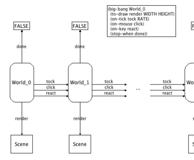
The big-bang form installs World\_0 as the initial WorldState. The handlers tock, react, and click transform one world into another one; each time an event is handled, done is used to check whether the world is final, in which case the program is shut down; and finally, draw renders each world as a scene, which is then displayed on an external canvas.
