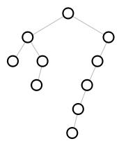
Uses the layout algorithm from *Tidier Drawing of Trees* by Edward M. Reingold and John S. Tilford (IEEE Transactions on Software Engineering, Volume 7, Number 2, March 1981) to lay out *tree-layout*.
