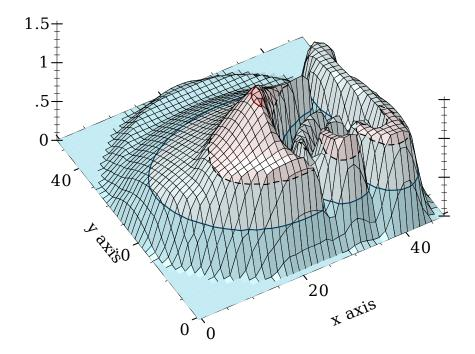
Notice that the plot's maximum height is above saturation (1.0). The tallest peak corresponds to the specular highlight (the shiny part) on the bomb. Specular highlights are one case where it is important to operate on oversaturated values without truncating them—until it is time to display the image.
