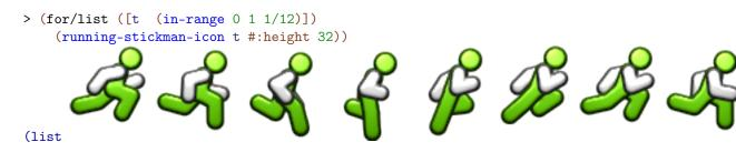
The stickman's joint angles are defined by continuous periodic functions, so the run cycle can be sampled at any resolution, or at any real-valued time t. The cycle is modeled after the run cycle of the player's avatar in the Commodore 64 game Impossible Mission.
