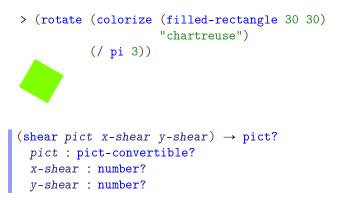
Shear's the *pict* by a factor of x-shear along the x-axis and by a factor of y-shear along the y-axis. The bounding box is inflated to contain the result. The result's ascent and descent are the same as *pict*'s.
