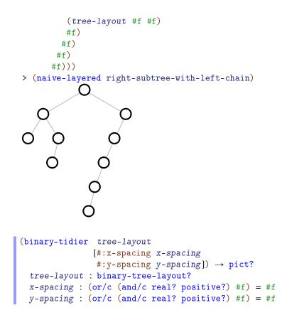
Uses the layout algorithm from *Tidier Drawing of Trees* by Edward M. Reingold and John S. Tilford (IEEE Transactions on Software Engineering, Volume 7, Number 2, March 1981) to lay out *tree-layout*.
