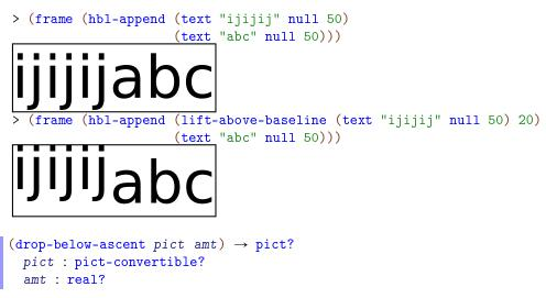
Drops pict relative to its ascent line, extending the bounding box height if necessary.
