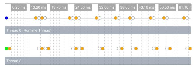
The problem is that most every arithmetic operation in this example produces an inexact number whose storage must be allocated. While some allocation can safely be performed exclusively without the aid of the runtime thread, especially frequent allocation requires synchronized operations which defeat any performance improvement.
