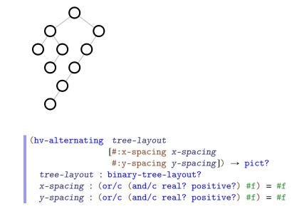
Uses the "CT" binary tree layout algorithm from A note on optimal area algorithms for upward drawing of binary trees by P. Crescenzi, G. Di Battista, and A. Piperno (Computational Geometry, Theory and Applications, 1992) to lay out tree-layout.
