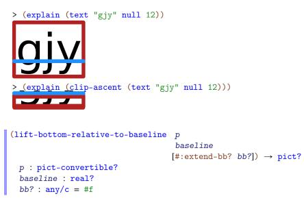
Lift the image in p such that the bottom of the picture is *baseline* above its baseline. If *bb*? is #f then the bounding box is unchanged, otherwise it is adjusted to fit the resulting pict.
