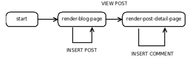
Each node (bubble) in this diagram corresponds to a request-consuming handler. As you might expect, we'll be using send/suspend/dispatch some more. Every arrow in the diagram will be realized as a URL that we generate with embed/url.
