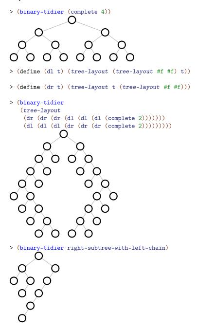
Uses the "CT" binary tree layout algorithm from *A note on optimal area algorithms for upward drawing of binary trees* by P. Crescenzi, G. Di Battista, and A. Piperno (Computational Geometry, Theory and Applications, 1992) to lay out *tree-layout*.
